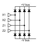
The AC power supply terminals can be connected to the alternator terminals (SHUNT), permanent magnet generator (PMG), auxiliary winding excitation principle (AREP) or external power supply.
