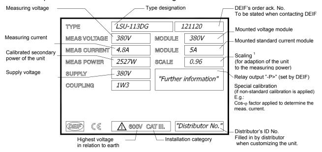
Note 1: Calculation of measuring power: voltage module x current module x scale  $x \sqrt{3} x \cos(\varphi) = measuring power$  "  $\sqrt{3}$ " is replaced by "1" for coupling 1W
