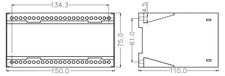
The LSU-113DG is designed for panel mounting, being mounted on a 35 mm DIN rail, or by means of two 4-mm screws.
