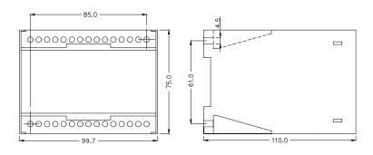
The RMV-132D is designed for panel mounting, being mounted on a 35 mm DIN rail, or by means of two 4-mm screws.
