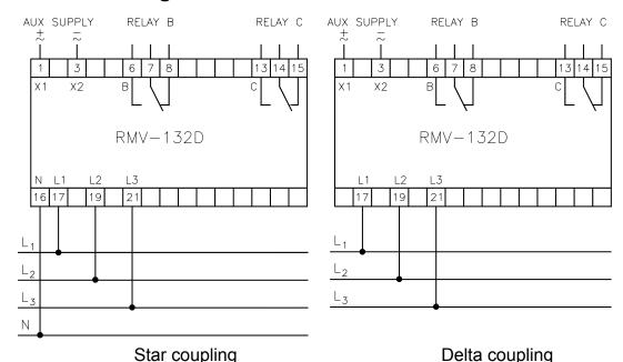
Please note the difference between relays for delta coupling and for star coupling. The coupling is stated on the label.
