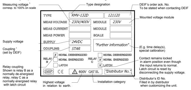
Note 1: Example of a label for an RMV-132D for delta coupling:
